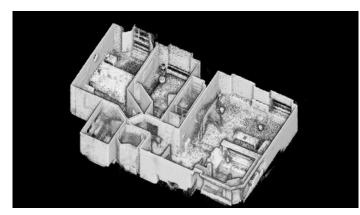
Capture and create real estate and commercial property floorplans with informative 360° panoramic photography for enhanced property surveys. 3D measurable information and imagery captured with the ZEB PANO uses the leading SLAM algorithm to automatically and accurately position panoramic photos and enables the creation of both 2D and 3D property floorplans.
